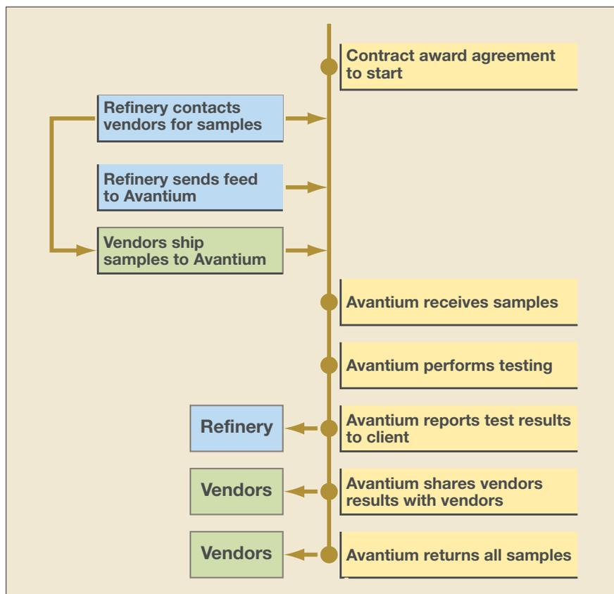
Figure 2 Workflow for third party catalyst testing
