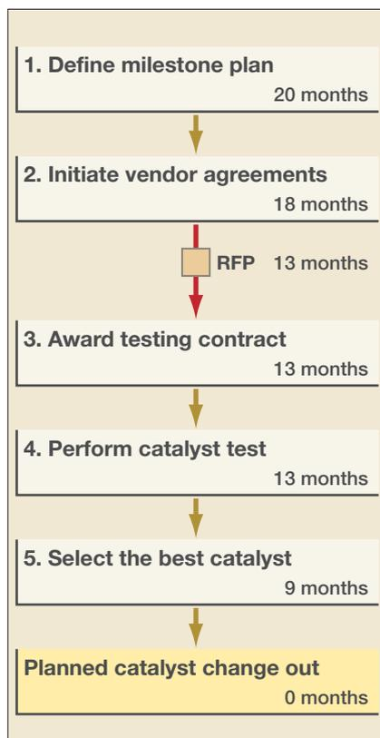
Figure 1 Milestones plan for catalyst testing and selection
